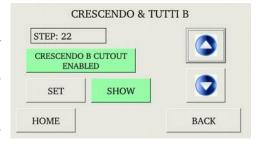
To view the stops registered on the second (B) Tutti I or Tutti II, press either Tutti piston. This will cause all associated stops programmed on the Tutti selected to turn on.
