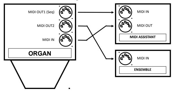
3. MIDI Transmission Channels MIDI information may be transmitted on several different channels simultaneously. This allows many channels of information to be sent through one cable and used independently from one another, similar to the way many television broadcasts can be sent through one cable. In order to receive the intended information, a MIDI device must be tuned to the same channel as the device that is sending the information.
