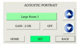
amount of gain available. To change the gain value, touch the gain value button to highlight it and then use the UP and DOWN buttons to change the gain value.
