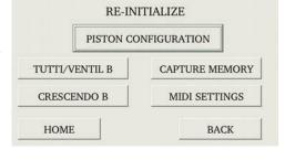
The Piston Configuration re-initialization includes all the Configure Piston settings. The MIDI Settings re-initialization includes all MIDI program change mapping. The Capture Memory re-initialization will reset the last available capture memory back to factory default registrations (*if applicable*).
