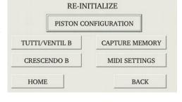
The Piston Configuration re-initialization includes all the Configure Piston settings. The MIDI Settings re-initialization includes all MIDI program change mapping. The Capture Memory re-initialization will reset the last available capture memory back to factory default registrations (*if applicable*).
